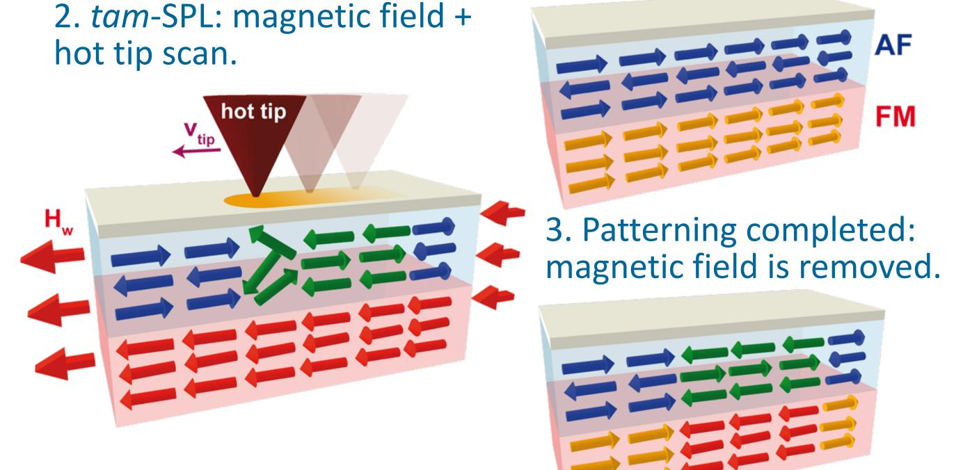
> Stabilization of 2D magnetic domains and 1D domain walls and 0D topological solitons via tam-SPL. Below, magnetic force microscopy images of the magnetic domains and domain walls.
