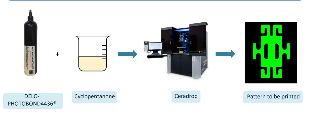
Dilution (1:3 by weight) was necessary to process the material. Cyclopentanone was chosen as diluent as it exhibits a sufficiently low viscosity ( $\eta$ =1.075 cP) and a not too high boiling point (T<sub>eb</sub>=130°C). The solution was transferred in a 10 pL Dimatix cartridge and mounted in the Ceradrop printhead.
