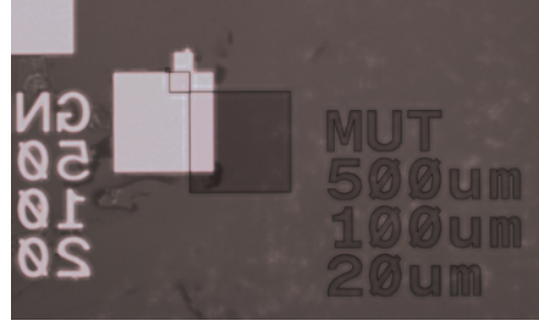
Figure 2: Lithographic test pattern showing the \approx 100 \mu\text{m} offset achieved through the back-side alignment via overview camera.
